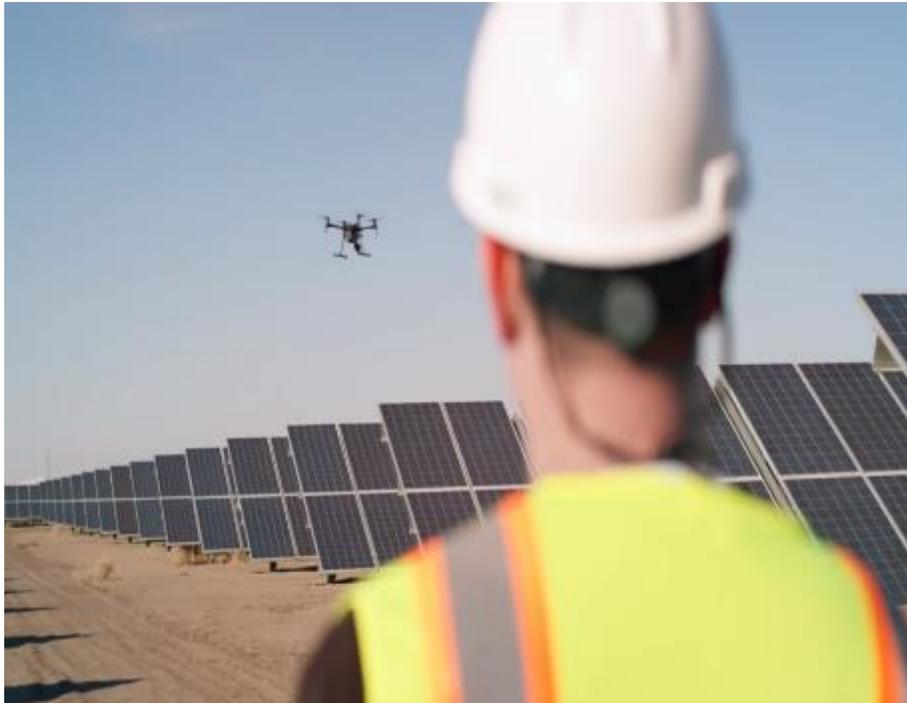
**Drone-based aerial thermography** to **detect significant temperature abnormalities** such as hot spots and hot areas on the Solar modules
